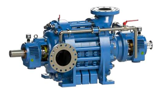
**Self-Balancing Multi –Stage:** SB pump units, which utilise non-friction, heavy duty ball and roller bearings to support the rotating element were successfully introduced to the market. As a result of this innovation, all standard balance disc centrifugal multi-stage pumps can now be converted from white metal bearing arrangements to the non-friction, heavy duty sliding roller bearings (SRB).
