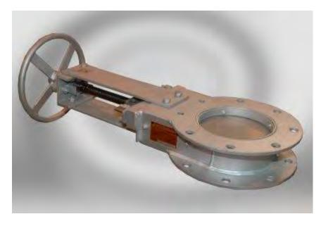
This wear ring ensures that contact of material with the sealing strip above the gate plate is minimized reducing wear and maintenance. The outlet port opening is larger than the inlet ensuring minimal chances of material hang-up.
